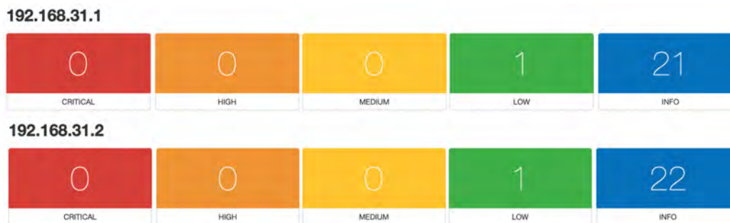
Figure 4.6. Cyber security vulnerabilities detected on the ECDIS system of the training ship Kapitan Gregorio Oca .
