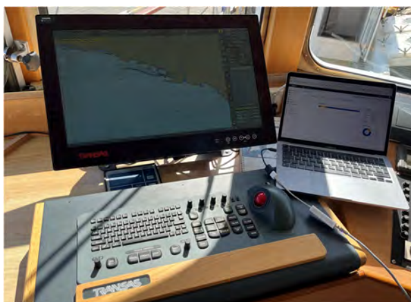
Figure 4.1. Cyber vulnerability scanning of the ECDIS system implemented on the training ship Kraljica mora .
